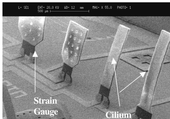
**Figure 6.** SEM of a fabricated haircell array with different heights and widths. The fabricated device has cilium length varying from  $600\ \mu\text{m}$  to  $1.5\ \text{mm}$ . The strain gauge is not apparent because of the top protective polyimide coating.
